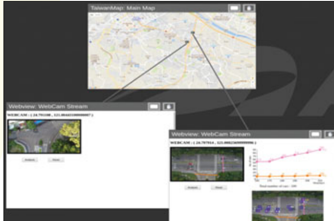
Figure 13. Screen shot of SAGE2 workspace of machine learning application for traffic monitoring. Multiple camera locations can be visualized and analyzed for the number of cars that pass a virtual gate set by the user.
