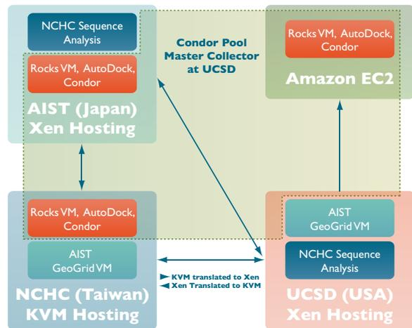
Figure 1: Three-site VM Portability Experiment. Each site authored a virtual machine (VM) and ran it at the other two sites. Conversions of VM formats were also managed
