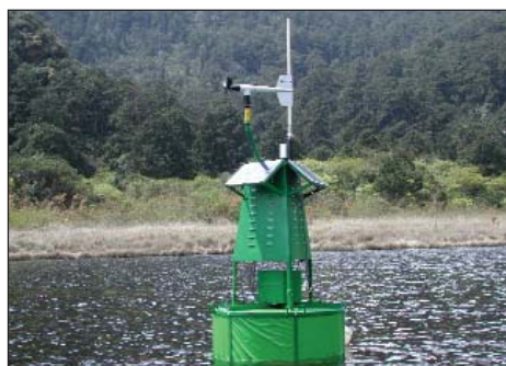
Buoy in Yuan-Yang Lake, Taiwan contains sensors and is integrated into the EcoGrid infrastructure.
