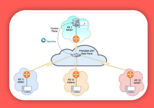
ONOS and the SDN-IP application provide peering between external networks and the Transit Network through BGP and the ONOS Intent framework.
