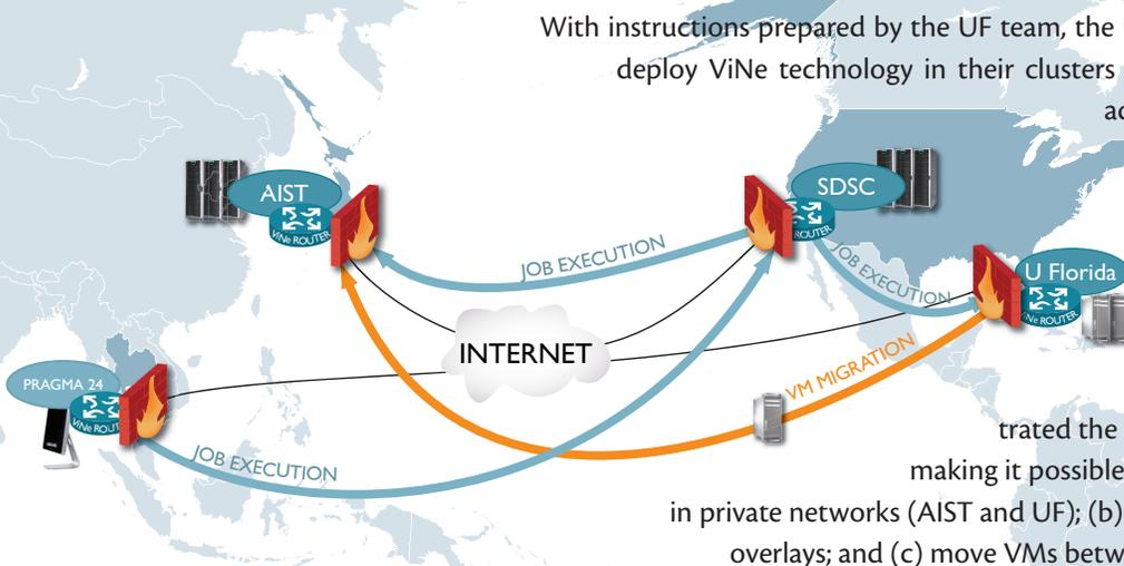
Figure 7. ViNe established the communication among physical and virtual resources on private networks at UCSD, UF, AIST, and PRAGMA 24 Workshop site (Thailand). This setup allowed live wide-area VM migration experiments and the deployment of a Condor pool across multiple countries.
