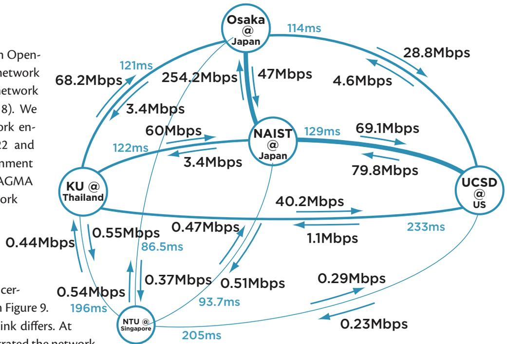
Figure 9. Network performance of the experiment environment
