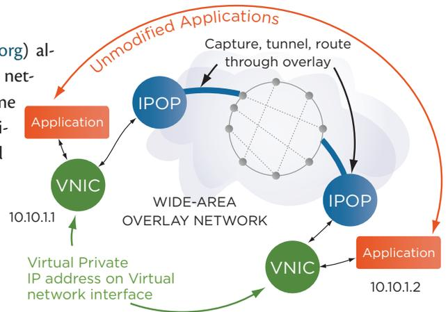
Figure 4. IPOP enables unmodified applications to connect over a self-configuring virtual private in a seamless manner. The key mechanisms used are: a virtual network interface to capture/inject packets, peer-to-peer overlay links through which virtual IP packets are tunneled, and overlay routing across wide-area networks.
