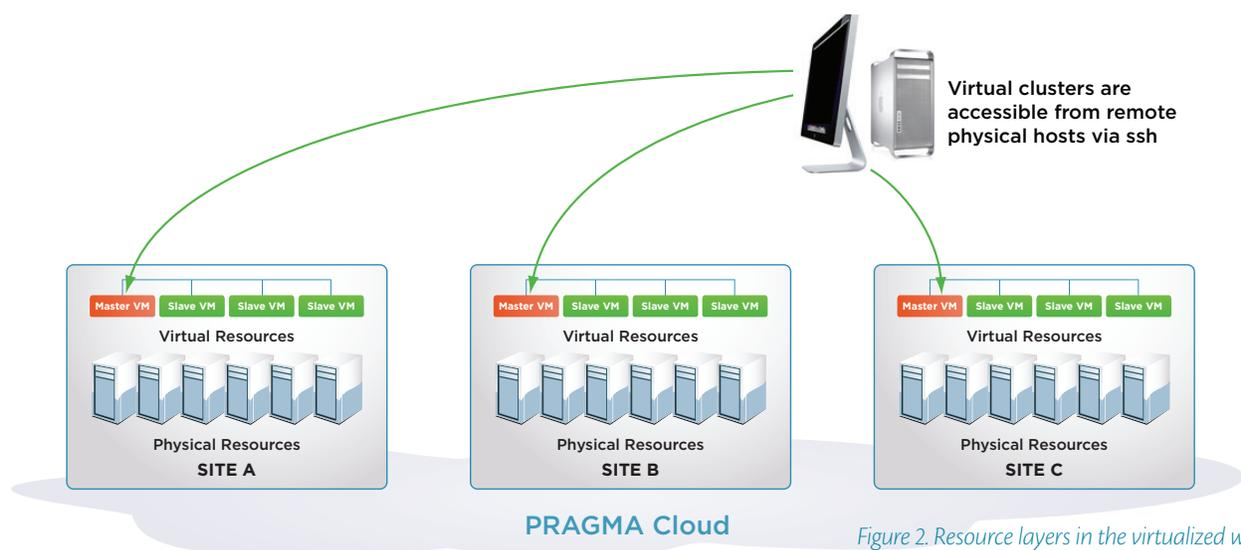
Figure 2. Resource layers in the virtualized workflow
