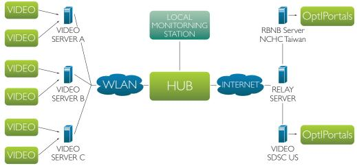
Figure 1: Setup for streaming live underwater cameras to OptIPortals
