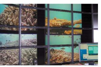
Figure 3:Tiled-display wall (TDW) at Calit2 (UCSD) showing data from underwater video cameras in Kenting (Taiwan) in real time using DataTurbine streaming data middleware.
